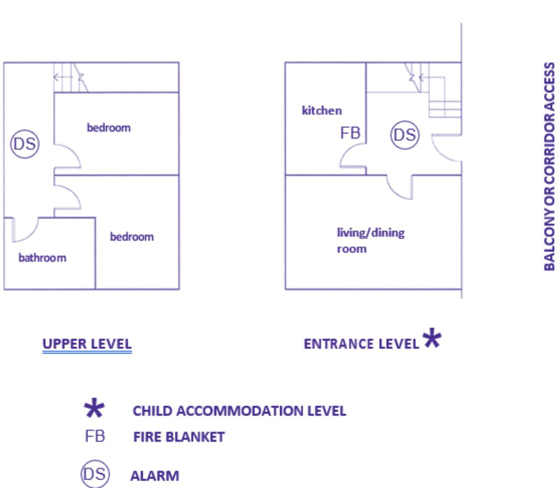
1. Install mains powered smoke alarms in ground floor entrance hall and upper floor level.
